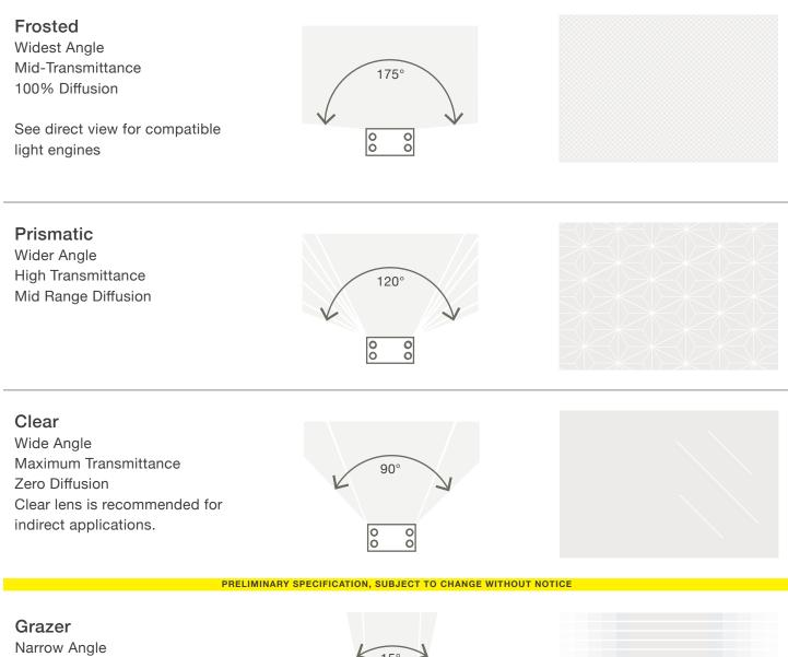
Narrow Angle 15° Collimation Optic Compatible with AT402
